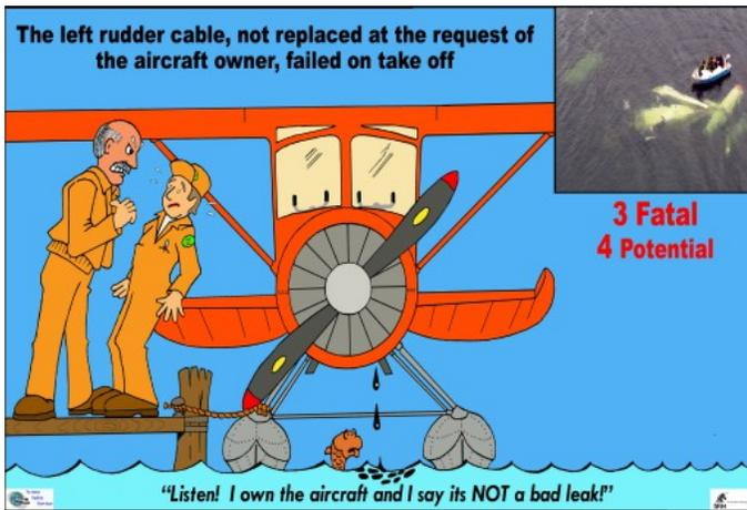
**Lack of Assertiveness** has been a contributing factor in way too many accidents. Looking at the cartoon takes us back to a fatal float plane accident up North many years ago. A conscious Aircraft Maintenance Engineer (AME) found a corroded rudder cable just inside the empennage on a routine annual inspection. He brought it to the attention
